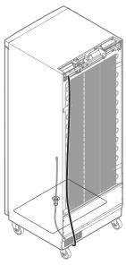
4. Close the sensor cable opening with the sealant provided.
