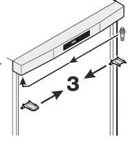
**4.** Transfer lower hinge bracket and cover plate to the opposite side.
