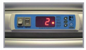
For manual defrost with this controller press the ▲ and ▼ buttons simultaneously for 5 seconds, together at the same time.
