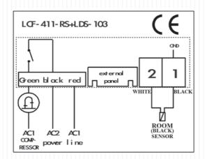
★ Room Sensor [black wire] need to connect to PIN 1 for ground purpose.
