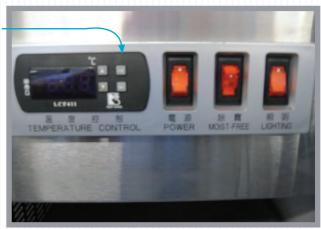
If this doesn't work then you may need to empty cabinet and leave off till fully melted. There may not be enough ventilation.
