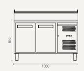
Allow min. 100mm clearance for instalation, all vents must be left clear
