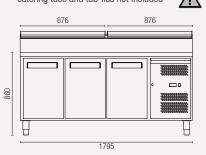
Allow min. 100mm clearance for instalation all vents must be left clear
