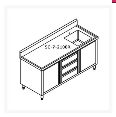
SC-7-2100R-H Cabinet with Right Sink. 2100mm wide cabinet is a great addition to commercial kitchen and hospitality workspace. Ideal for open kitchens with punched bowls, 90mm diameter drain hole. 1.2mm top & frame built from SUS304 grade stainless steel with 2 doors and 3 drawers. Pre-mounted with all welded joints.
