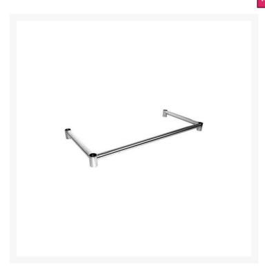
LB7-1500/A Leg Brace is a stainless steel commercial leg brace with 1.2mm SUS304 (18/8) and BA finish. Comes with 38 diameter 1.2 mm tube. It measures 490mm wide x 590mm deep. Leg brace must be used for stability when no undershelf is required.
