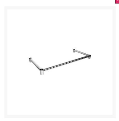
LB7-2100/A Leg Brace is stainless steel commercial leg brace with 490mm width x 590mm depth. Leg brace must be used for stability when no undershelf is required. Fabricated with 1.2mm SUS304 (18/8) grade material with BA finish. Comes with 38 diameter 1.2 mm tube.
