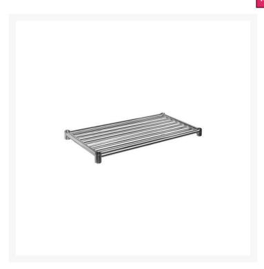
PRU7-2100/A Pot Undershelf is SUS304 grade stainless steel built, 1.2mm thick, BA finish pot undershelf. 25 diameter inner tubes crafted with 1mm stainless steel with 40mm spacing. 38 diameter outer frame tubes built with 1.2mm S/S. It is a perfect choice for commercial workbench and sinks.
