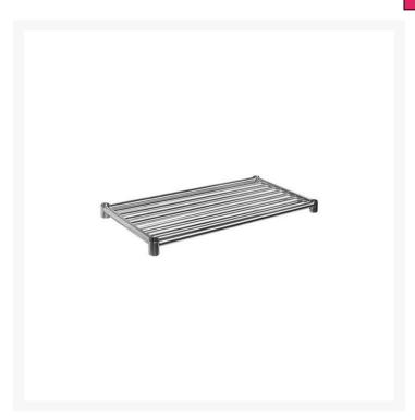
PRU7-2400/A Pot Undershelf. SUS304 grade 1.2mm thick stainless steel built with BA finish. Perfect choice for commercial workbench and sinks. 25 diameter inner tubes crafted with 1mm stainless steel with 40mm spacing. 38 diameter outer frame tubes built with 1.2mm S/S.
