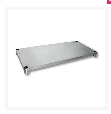
SUS6-0600/A Solid Undershelf is an ideal solution for storage issues in commercial kitchen workbenches and sink. Constructed with 1.2mm thick SUS304 grade stainless steel with a hairline finish. Special U channel reinforcements under to suit the bench type & size. U channel width increases as the bench size increases.
