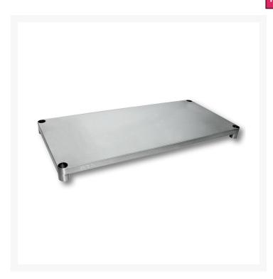
SUS6-0900/A Solid Undershelf for commercial workbenches and sink. Fabricated with 1.2mm thick SUS304 grade stainless steel with a hairline finish. Special U channel reinforcements under to suit the bench type & size. U channel width increases as the bench size increases.
