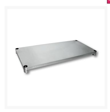
SUS6-1200/A Solid Undershelf is an excellent option for storage extension in commercial workbench and sink. SUS304 grade stainless steel built with a hairline finish. 1.2mm thick S/S with special U channel reinforcements under to suit the bench type & size. As the bench size increases so do the U channel width.
