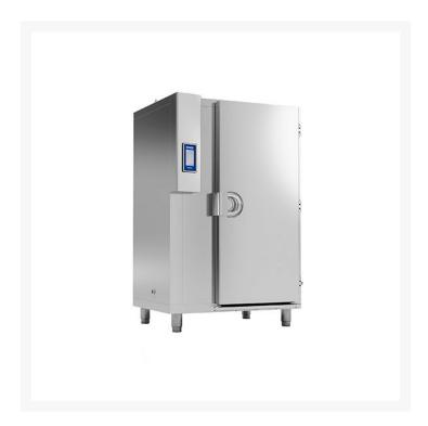
Irinox-MF-130.2 ST is the standard caster out rack in version, a tray capacity of 1(GN 2/1), can make 130 kilograms of ice, a 90 to negative 18 degrees centigrade temperature range, with 1.1kW peer hour energy consumption, a refrigerant gas R452A, an ambient rating of 32 degrees centigrade, equipped with HACCP control software.
