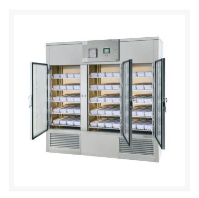
Arrowsmith and Grant AG308BP Glass Door Blood Refrigerator has a dimension of 2065mm (W)  $\times$  805mm (D)  $\times$  2000mm (H), can hold 676  $\times$  450ml blood packs, temperature range of 2.5 to 5.5 degrees centigrade, and refrigerant gas of R507.
